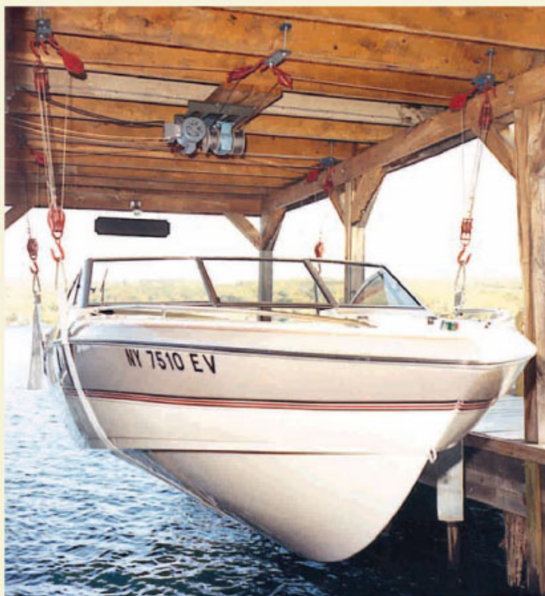
Boat House Lift with Adjustable Slings
